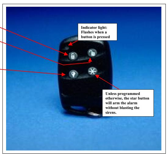
Remember: When pressing a button it is necessary to hold the button down for one (1) second for signal to be sent. This feature avoids unintentional operations from remote.
